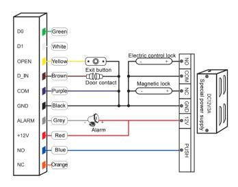
Note: The door contact and alarm function are optional
